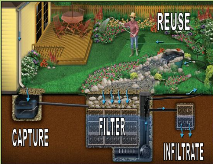
Diagram of an Aquascape™ Rainwater Catchment System
